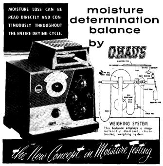
A combination drying unit and Precision Balance, this instrument can be used for solids or liquids, and shows the percentage of moisture directly to plus or minus 0.1%.
